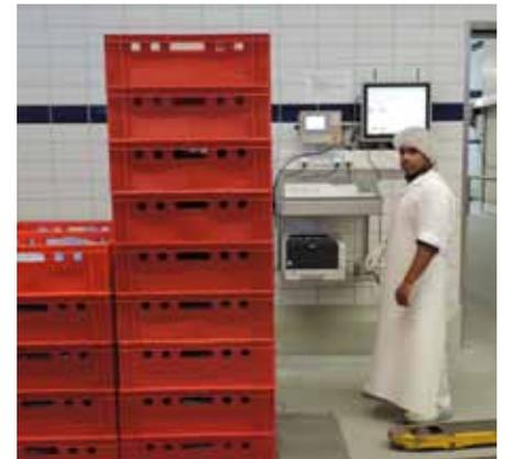
**The pallet is weighed at the disassembly exit and is given a barcode label.**
